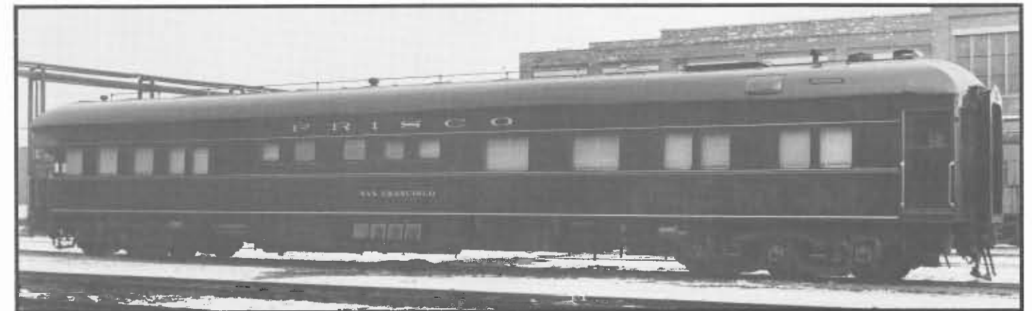
Right side view, Frisco Business Car San Francisco, with turtleback roof design West Springfield Coach Shops, December 21, 1956 Frisco photo
